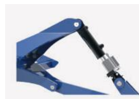
Hydraulic adjustment of working depth - STANDARD
