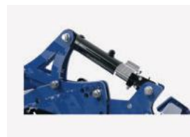
Hydraulic adjustment of working depth - OPTION
