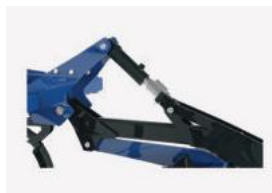
Hydraulic adjustment of working depth - STANDARD
