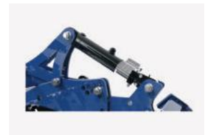
Hydraulic adjustment of working depth - OPTION
