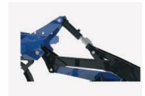
Hydraulic adjustment of working depth - STANDARD
