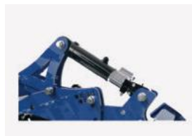
Hydraulic adjustment of working depth - OPTION
