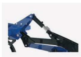
Hydraulic adjustment of working depth - STANDARD
