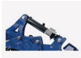
Hydraulic adjustment of working depth - OPTION
